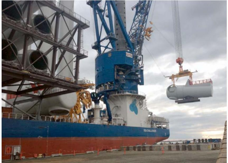
88 metre turbine towers being secured to the deck of the Sea Challenger. The spiral wraps seen on the towers are temporarily fitted to reduce vortex forming (which could cause instability) above the towers during transportation.
